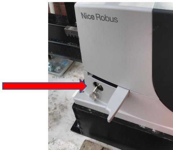
3. The gate may now be rolled open or closed. The clutch should now be re-engaged and the key returned to the key box.
